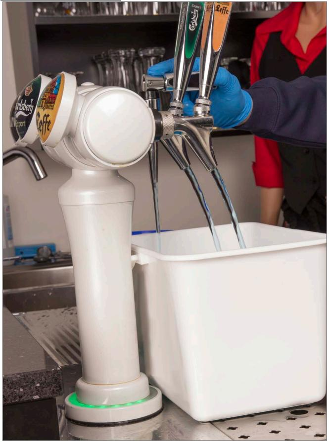
8. Rinse and fill the cleaning bottle with cold, clean water and connect the keg couplers.
